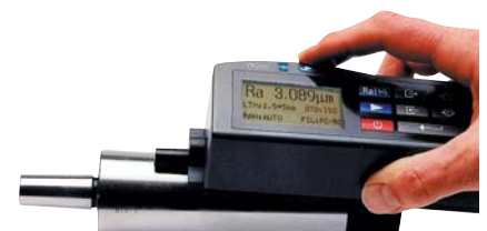
Extra start button easy accessible for hand held operation
