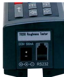
Data output RS-232 and charger input at back side
