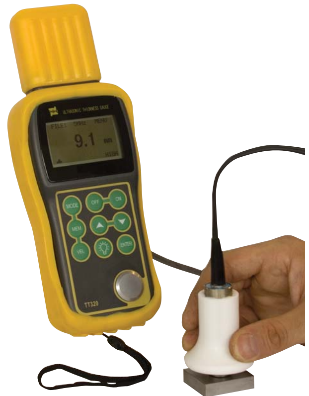
Special high temperature transducer
